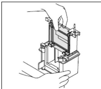
**Slide Gel Cassette Sandwiches and Electrode Assembly Into the clamping frame.**
