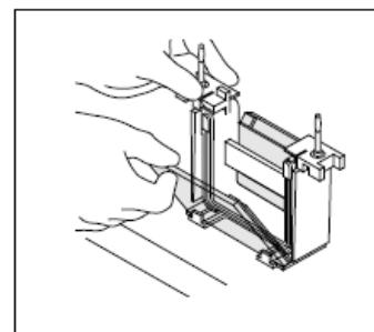
Place Gel Cassette Sandwich into the Electrode Assembly with the Short Plate facing inward.
