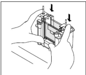
**Press down on the Electrode Assembly while closing the two cam levers of the Clamping Frame.**
