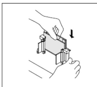
Slide the two plates into the Casting Frame keeping the Short Plate facing front.
