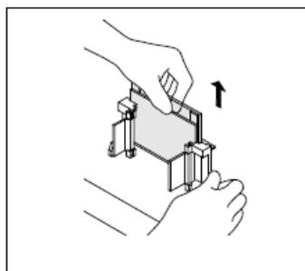
Remove the Gel Cassette Sandwich from the Casting Frame.
