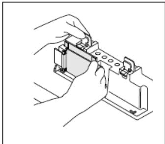
**Secure the Casting Frame in the Casting Stand by engaging the spring loaded lever.**
