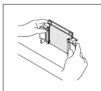
Lock the pressure cams to secure the glass plates.
