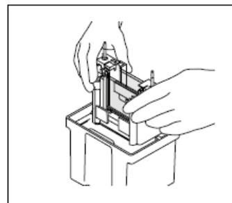
**Lower the Inner Chamber into the Mini Tank.**
